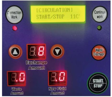
Internationally normal ATF changing process is CONNECTING WORK. It means that connect machine two line to any of oil cooler line and then connect in and out hose with direction and then ready to operation.
