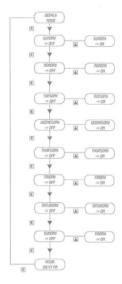
Use this menu to setup dosing activity on daily base, duration and starting time. Press "E" key to scroll, press "UP" (choose digit) and "RIGHT" key (next digit).
