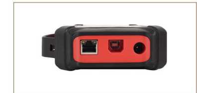
LAN/WAN Port, Data I/O port & DC-IN Power Jack
