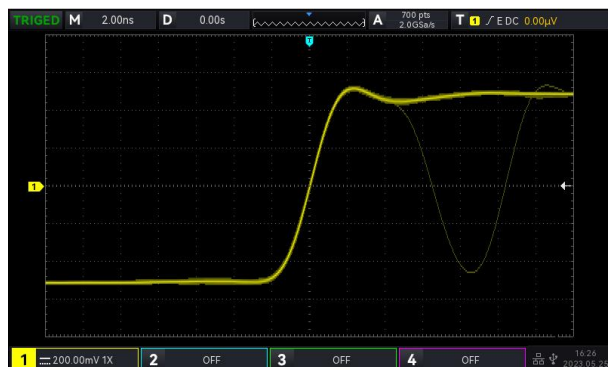
Use the innovative digital signal parallel processing technique, normal sampling up to 150,000wfms/s, capture the accidental signal. (In Fast Acquire mode, the capture rate up to 500,000 wfms/s.)
