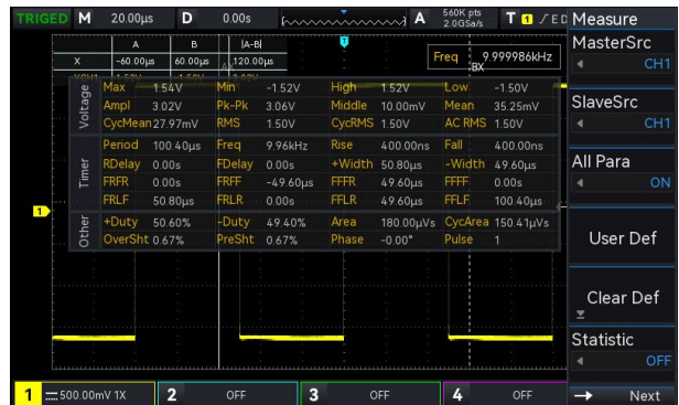
When the Cursor is opened, the waveform in cursor area can process the parameter measurement. It is convenient for user to process the waveform measurement in the specified area, it enhances the flexible and operability for the measurement area.
