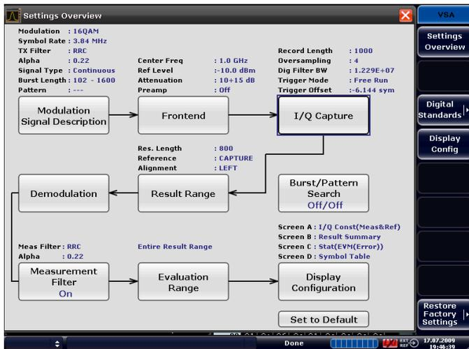
Based on the description of the signal to be analyzed (e.g. modulation format, continuous or with bursts, symbol rate, transmit filtering), the R&S®FPS-K70 option supports users in automatically finding useful settings.
