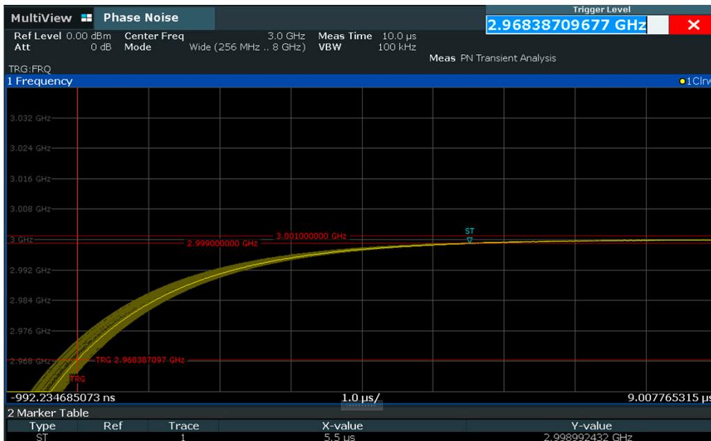
Transient response of a synthesizer in persistence mode. The horizontal red line shows the frequency trigger threshold, the vertical line the trigger offset. The bright yellow trace is the current measurement, the dull yellow traces show all previous measurements.
