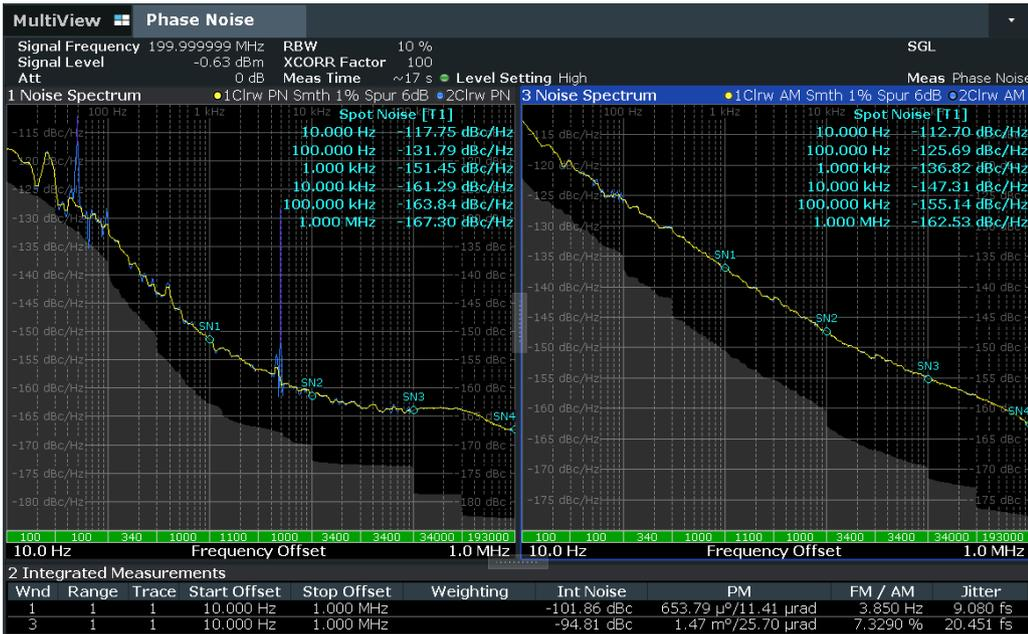
The R&S®FSPN can measure phase noise and amplitude noise simultaneously. The gray area below the traces shows the cross-correlation gain of the R&S®FSPN.
