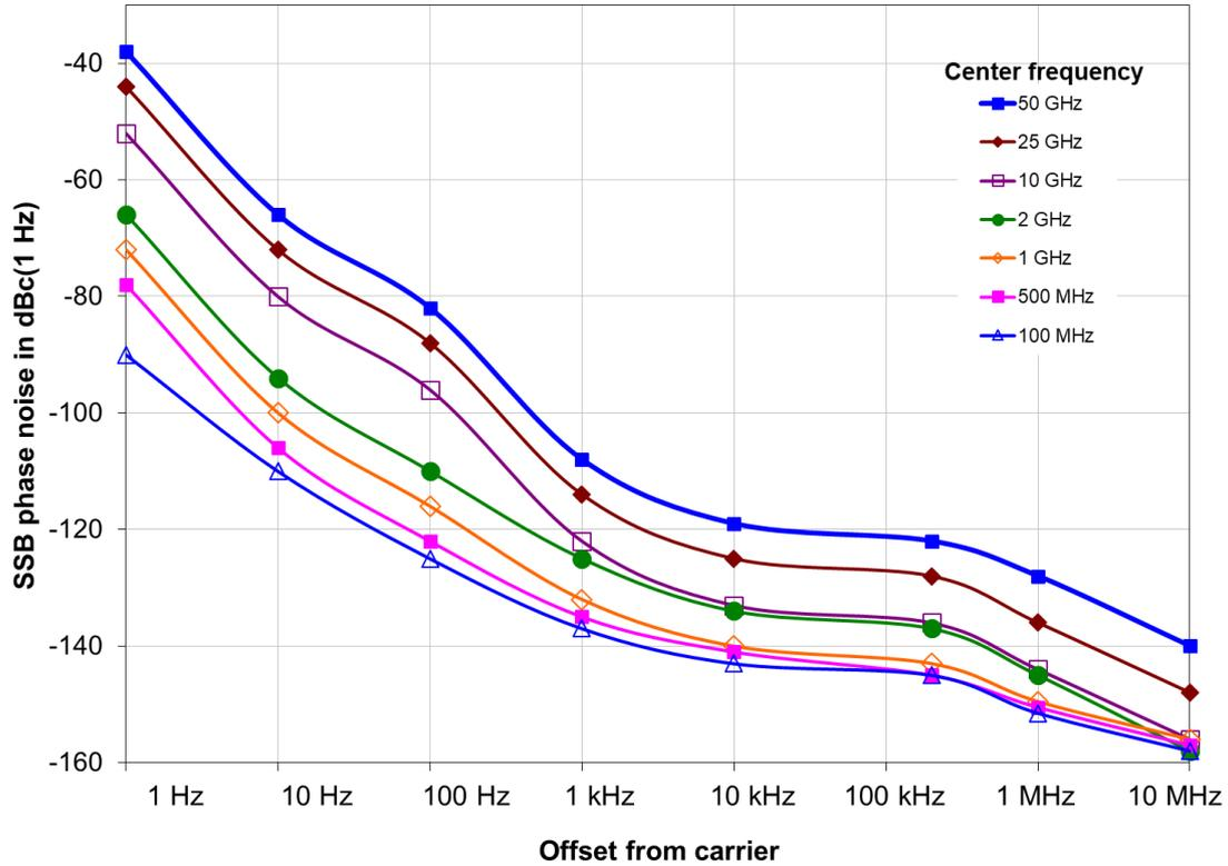
Typical phase noise at different center frequencies in spectrum analyzer mode (with R&S®FSMR3-B4 option for offsets  $\leq 10$  Hz)
