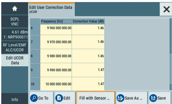
After the user correction table has been activated, the R&S®SMA100B adapts its output power to compensate for the frequency response of the RF cable.
