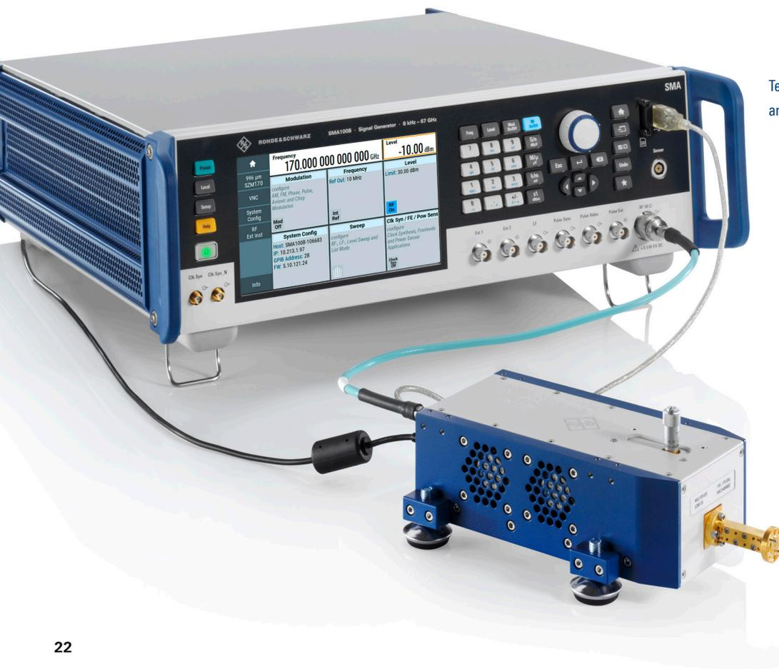
Test setup consisting of the R&S®SMA100B and the R&S®SzM170 frequency multiplier
