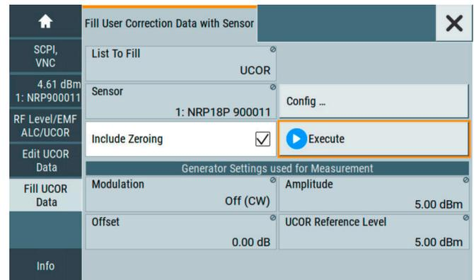
The measured level correction values are stored in a table with the user-selected frequencies.
