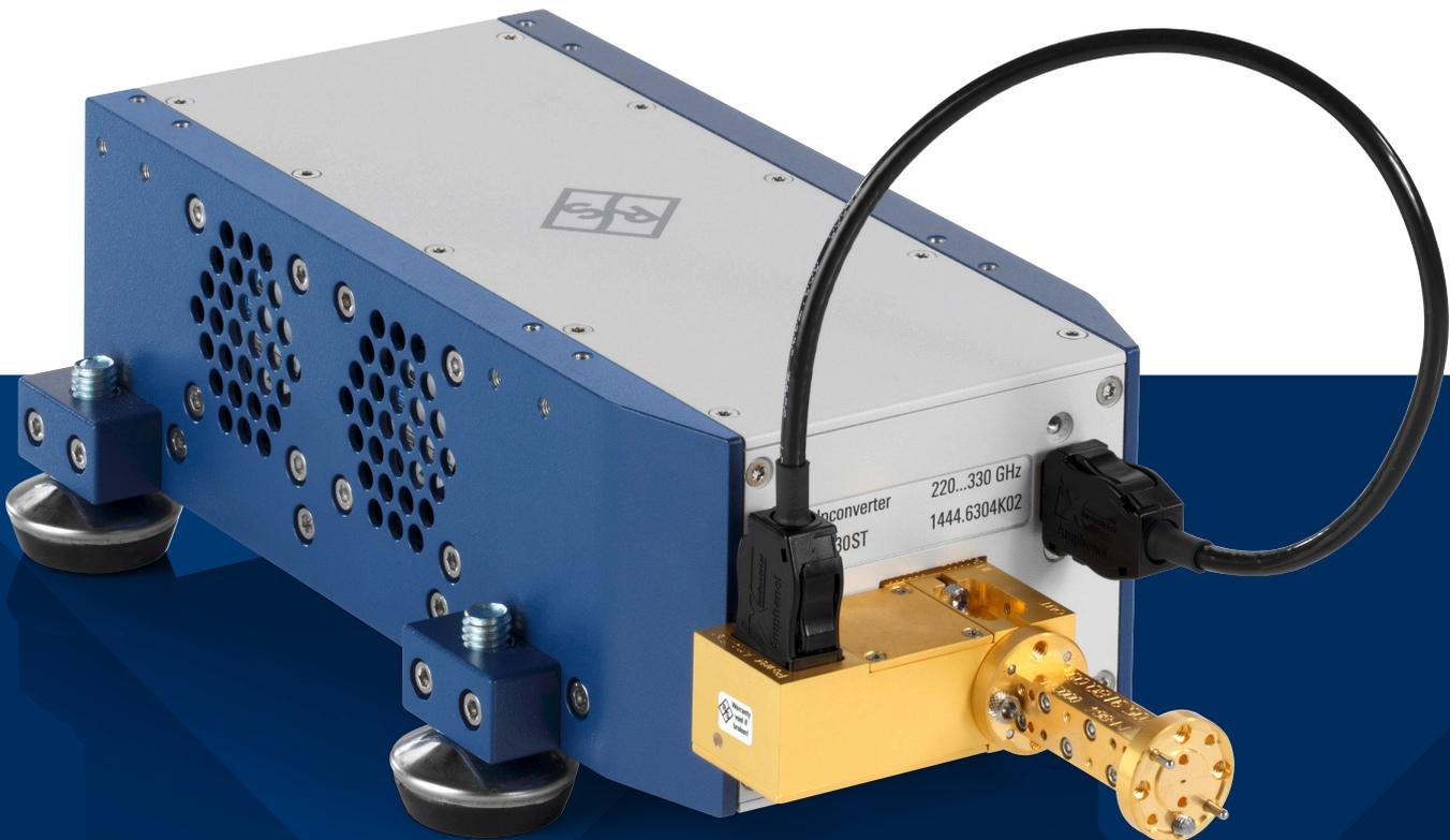
The main component of the R&S®FC330 frequency converters is a subharmonic mixer. In general, a mixer consists of two input ports and one output port. The two input signals are mixed so that the output signal frequency is either the sum or the difference of the source frequencies.
