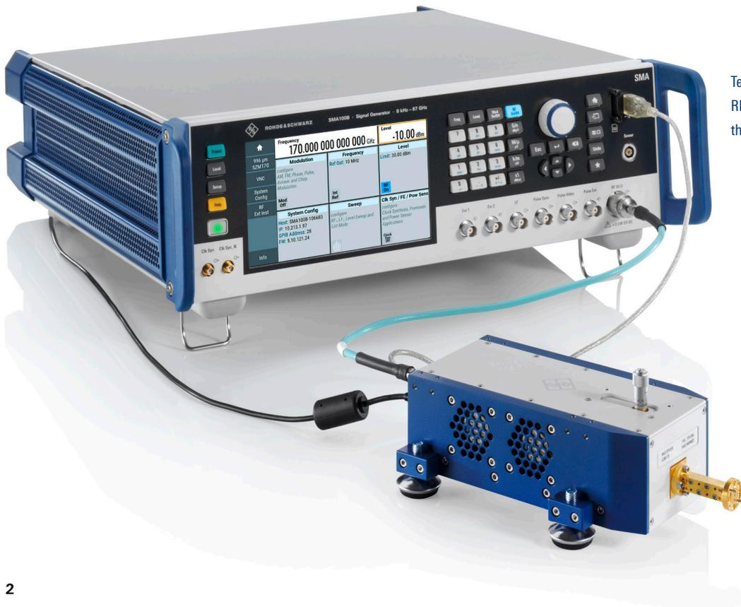
Test setup consisting of the R&S®SMA100B RF and microwave signal generator and the R&S®SZM170 frequency multiplier
