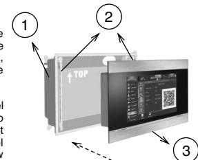
**IV.** Finally, the touch panel is placed in the mounting box by moving in the direction of the dashed arrow. Then it is screwed to the mounting frame through the screw slots on the 4 corners of the panel. Magnetic materialised lath with 2 horizontal holes on it should be attached to the lower part of the panel and the other one is attached to the upper part of the panel and the mounting process is completed.
