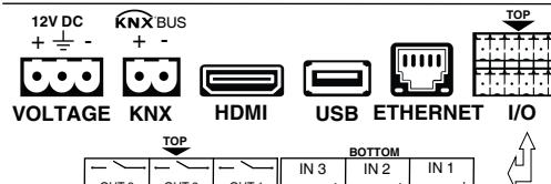
**Voltage:** Interra touch panels are powered by a special 3-pin green industrial special connector with 12V DC voltage. Pin indications are written on the plastic case. The cables of the 12V power supply must be plugged by the polarity.
