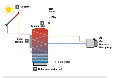
Domestic hot water systems with decentralised, germ-free water heating. Higher operating temperatures for the hot water enable an improved solar yield in comparison with boiler systems. The domestic hot water heating is conducted hygienically according to the continuous flow principle in maintenance-free operation. Partial solar space heating for countries with solar radiation above 1000 W/m<sup>2</sup>.
