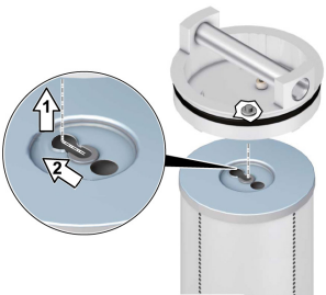
Fig. 7: Attaching the filter element
