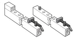
Or use a drilled  $2 \times 4$  with a block of wood secured at one end.
