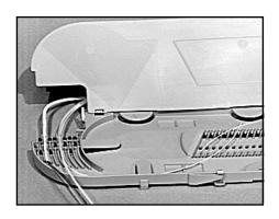
6.04 Place the splice assembly tool close to or on top of the splice tray. Match the orientation of the tool to that of the splice holder or tray whenever possible.
