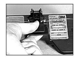
4.10 Remove the Fibrlok Splice from the assembly tool by first removing the fibers from the foam retention pads and then lifting the splice from the splice holding cradle.
