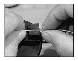
4.02 Grasp the coated fiber about .25 inches (6 mm) from the bare glass and move the fiber end onto the fiber alignment guide on the assembly tool such that the end is resting on the alignment guide outside of the splice.
