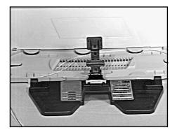
6.05 Remove the minimum amount of fiber required for fiber preparation and splicing. Remove less than one loop if possible.
