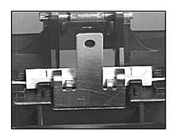
5.03 Slide the bottom of the cap lifter inward until it is in a vertical position, lifting the splice slightly out of the cradle.
