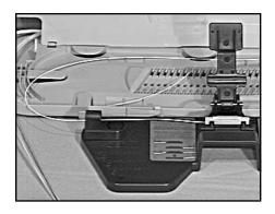
6.06 Prepare fibers and complete splice as described in Section 3 and 4.
