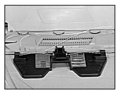
6.07 Carefully lay the splice on top of the holder without securing the splice into the holder.
