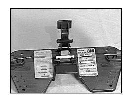
4.09 Pivot the handle of the Fibrlok Assembly Tool down until it contacts the cap of the Fibrlok Splice. Squeeze the handle of the assembly tool as shown in order to close cap and actuate the splice. When possible, secure the tool to a work surface for added support. A snap sound will be heard when the splice is actuated.
