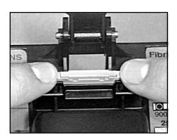
2.05 If using the Fibrlok 2501 Assembly Tool, rotate the toggle arms for the appropriate fiber size.
