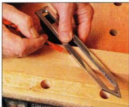
The angled arm is perfect for marking mitres
