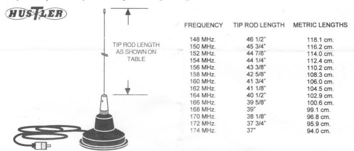
Insert a reliable S.W.R. bridge in the coax line and record the S.W.R. at the high, center, and low edge of the bands. If the S.W.R. is lowest at the high end, lengthen the tip rod in 1/4" length increments; if it is lowest at the low end, shorten the tip rod. Should the tip rod need to be shortened, do so by grinding the rod from the bottom end. Be sure to remove all burrs from the rod before reinsertion.
