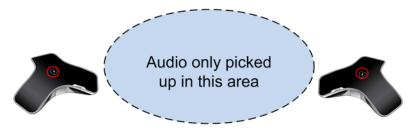
If two RealPresence Group Series Microphone Arrays are hooked up, audio is only picked up in the area that intersects the two beams (pointing opposite the mute button on each microphone).
