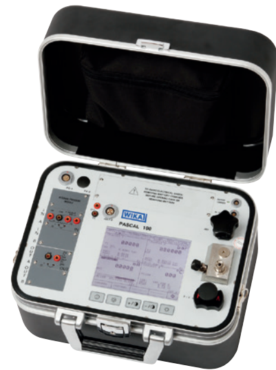
Hand-held multifunction calibrator, model Pascal 100
