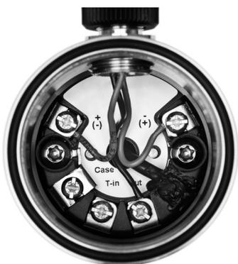
A Teach-In is necessary when the dielectric constant ( $\epsilon_r$ ) is  $< 2$  or a medium is hard to detect as present or not, e.g. when yogurt sticks to the sensor tip. Teach-In can be done directly with the product by using the teach terminals in the housing.
