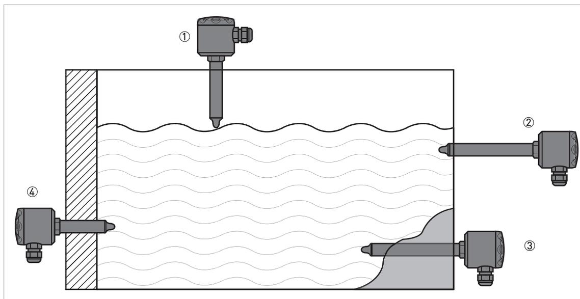
Figure 3-1: Possible applications for sliding connection
